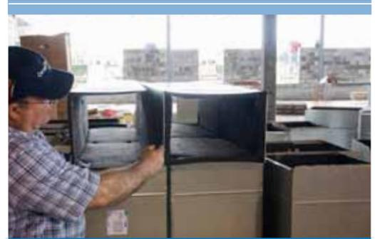
Commercial Air fabricated 2,500 feet of spiral and rectangular ductwork in their shop for the support rooms of the facility.
