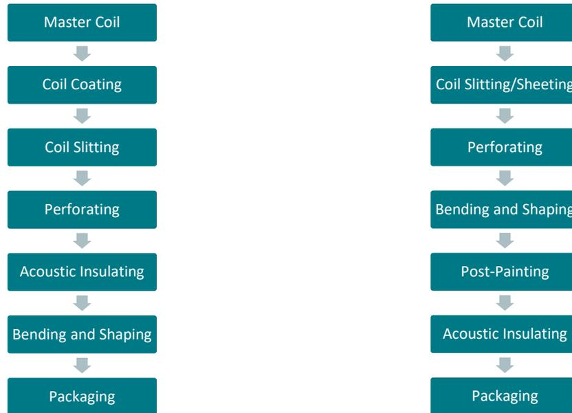
Figure 1: Typical steel specialty product manufacturing process, coil-coating (left) & post-painting (right)
